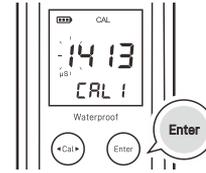
1.5 Press the **Enter** key, the tester begins the calibration. When the reading has stabilized, the display will show **End**. Calibration is completed.
